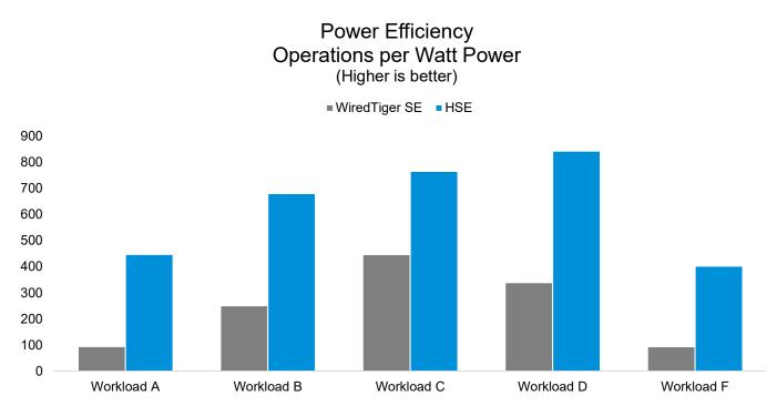
Figure 4: Power Efficiency Comparison of HSE vs. WiredTiger Storage Engines
